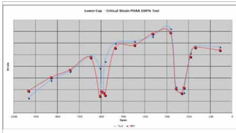
Figure 2: Physical measurements and finite element analysis predictions for strain on the lower spar cap
