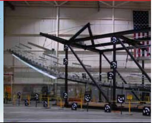
The Global Observer is an unmanned aircraft with the wingspan of a Boeing 767 but less than 10% of the weight designed to provide communications and sensing for flights lasting up to one week at up to 65,000 feet. With a maximum wing loading of only 3.5 pounds per square feet, the wingtip deflects greater than 22 feet at its design limit load.
