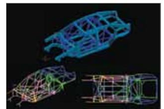
Integrated shell and cage design : optimisation for torsional stiffness
