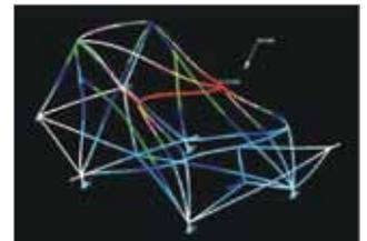
Integrated cage and shell design – simulation of lateral hoop test
