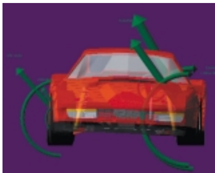
Control actions of a vehicle driver such as steering, braking, accelerating, gear shifting, and clutching for a variety of maneuvers can be simulated with ADAMS/Driver.
