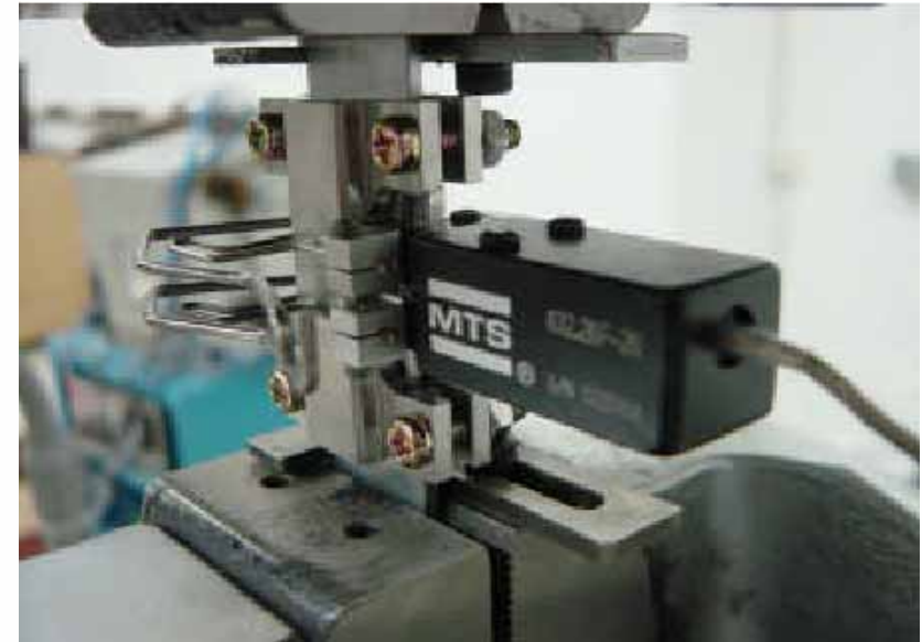
Example of Anti-buckling restraints for thin plate specimen
