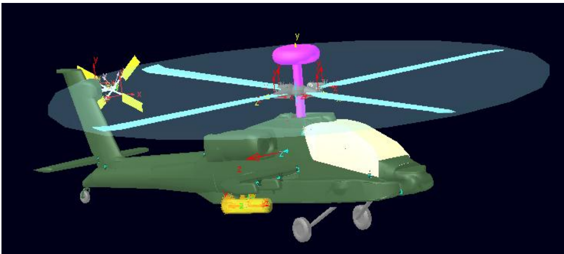
Figure 6. Apache-D Model with M261 Rocket Launcher and a Single Rocket
