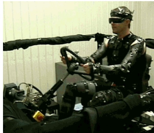
Figure 2. Test rig to simulate actual working conditions of the off-road heavy vehicle. Operator is rigged with photo reflective markers used to capture the motion during the exercise. Input to the rig is through a 6 dof moving platform.
