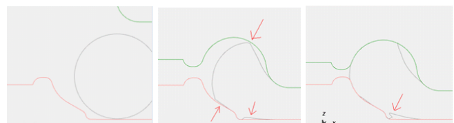
Figure 6: Progression of Fold in Rougher – Simulated
