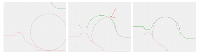
Figure 6: Avoidance of Fold in Rougher - Simulated
