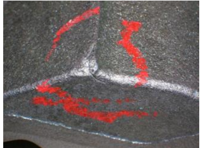
Figure 2: Lap that occurred during physical try-out
