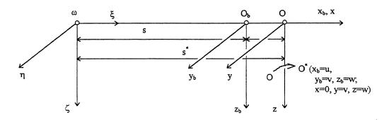
Fig. 2-1. The position of the wheelset and the vehicle body
