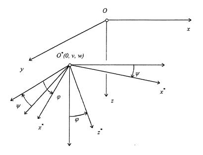
Fig. 3-1. The displacement of the wheelset
