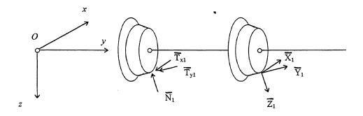
Fig. 4-1. The velocities and forces in the right hand contact point
