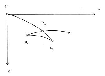
Fig. 3-4. The relation between  $\nu$  and  $\phi$  in the neighbourhood of a double-contact point
