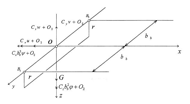
Fig. 2-2. The forces which are applied at the wheelset
