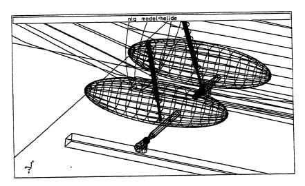
It creates an action-reaction force acting between two given points to connect, and an appropriate spring-damper geometry to show its position; no part (and hence no mass) is associated with this element.
