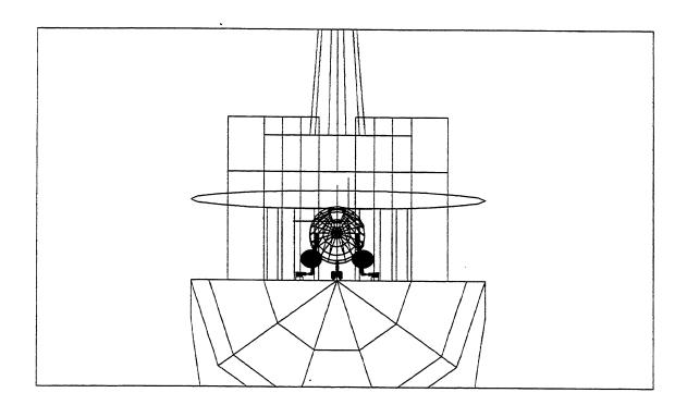
No attempt has been done to "logically parametrize" the helicopter topology: e.g. the connectivity and geometry of the Main Landing Gear are those of a given type of helicopter (NH90 at present); different helicopter models will have to be created using different macro files, owing to the probably different coordinate systems, number of parts, landing gear geometry and DOFs.
