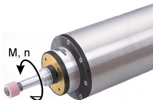
Figure 12: spindle with inner torque and gyroscopic characteristic
