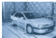
Anechoic chamber with chassis dynamometer
