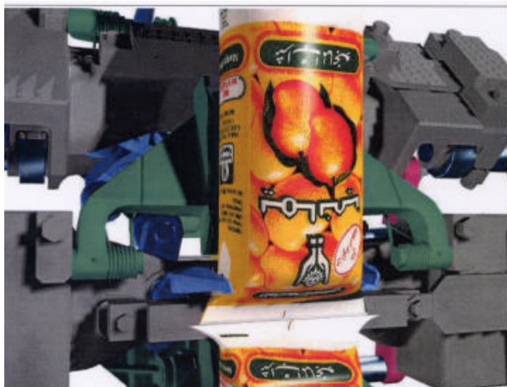
Fig. 5 The printed image is kept in position by the folding flaps (blue).
