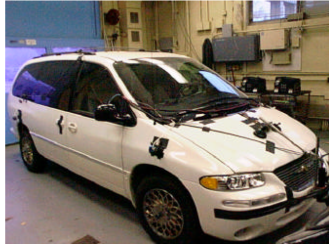
Figure 3: Instrumentation for the AWD minivan Dynamic tests
