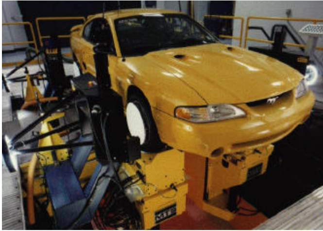
Figure 1: Kinematics and Compliance testing machine
