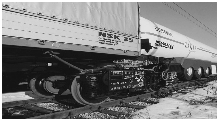
Fig.1. The view of the fragment of the bimodal train consisted of rigid car bodies and flexible cistern. Courtesy by "Research Institute of Rolling-Stock Industry", Poznan.
