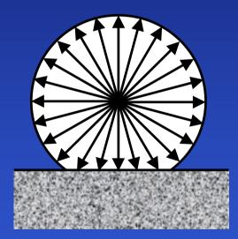
The radial stiffness is defined by a multiple radius contact wheel
