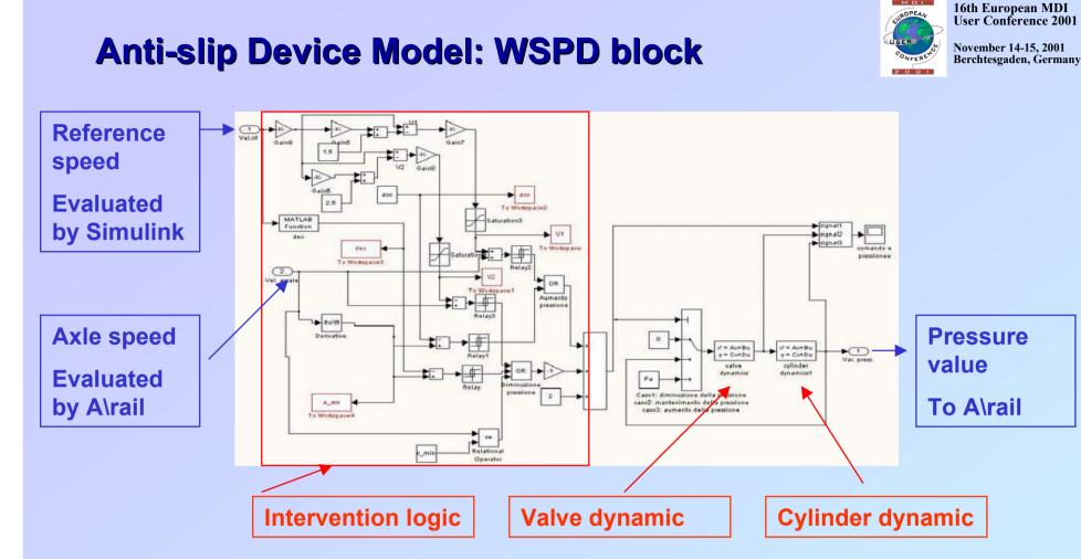
We took in account the air brake dynamics i.e. the pressure delay in reaching the sought value. Knowing the pressure values in the brake cylinders a function calculates automatically the correspondent value of braking couples that is applied to the wheelsets and these values are the input data for the Adams/Rail block.
