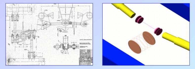
We considered useless an accurate modelling of the traction system. This element, in fact, gives a force that acts only in the longitudinal direction so it has been decided to model it inserting a spring whose axis is parallel to the X axis (the rail axis) with a very high axial stiffness and an insignificant transversal stiffness.
