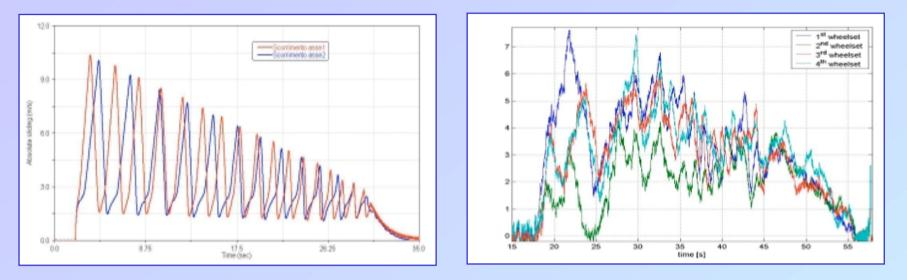
The noise present in the experimental graphics is mostly due to the high sampling frequency of the measuring instruments, while the longer time step characteristic of the Adams simulation acts like a low-pass filter and smoothes discontinuities.
