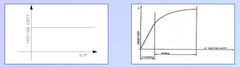
With such a contact model, there is a shorter braking distance in case of wheels blocked and complete sliding rather than in a case in which we avoid this situation using a wheel slide protection device.
