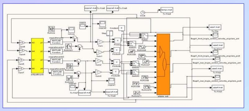
Adams/Controls Simulink block reproduces wagon mechanical behaviour, whose inputs are the braking couples and whose outputs are the angular velocities of the four wheel-sets
