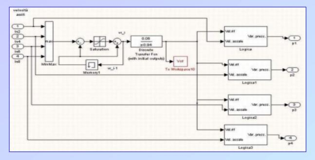
We consider as reference speed the greatest among the four axles velocities unless the deceleration overpasses a certain threshold; in this case we reconstruct the reference velocity integrating the threshold value.
