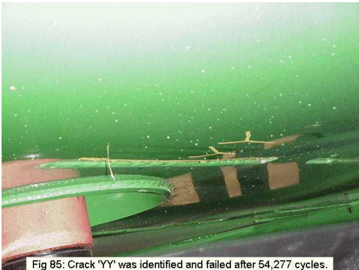
Figure 9 – Failure on Centre Cutter Lower Deck Near Cutter Shaft Bowl
