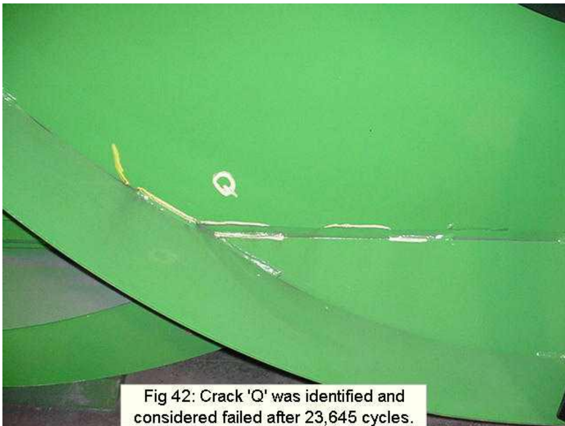
Figure 12 – Failure on Wing Cutter Lower Deck
