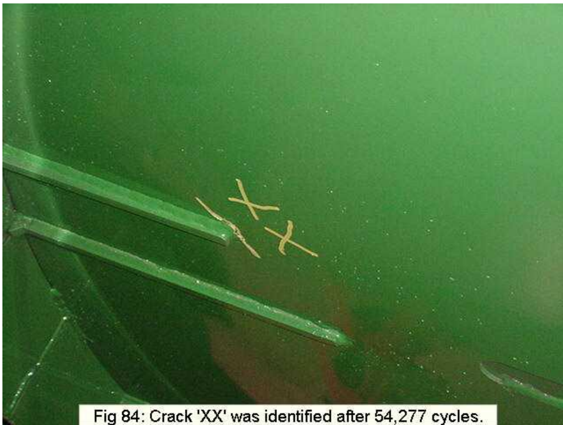
Figure 7- Failure on Centre Cutter Lower Deck at Hitch Support Plates
