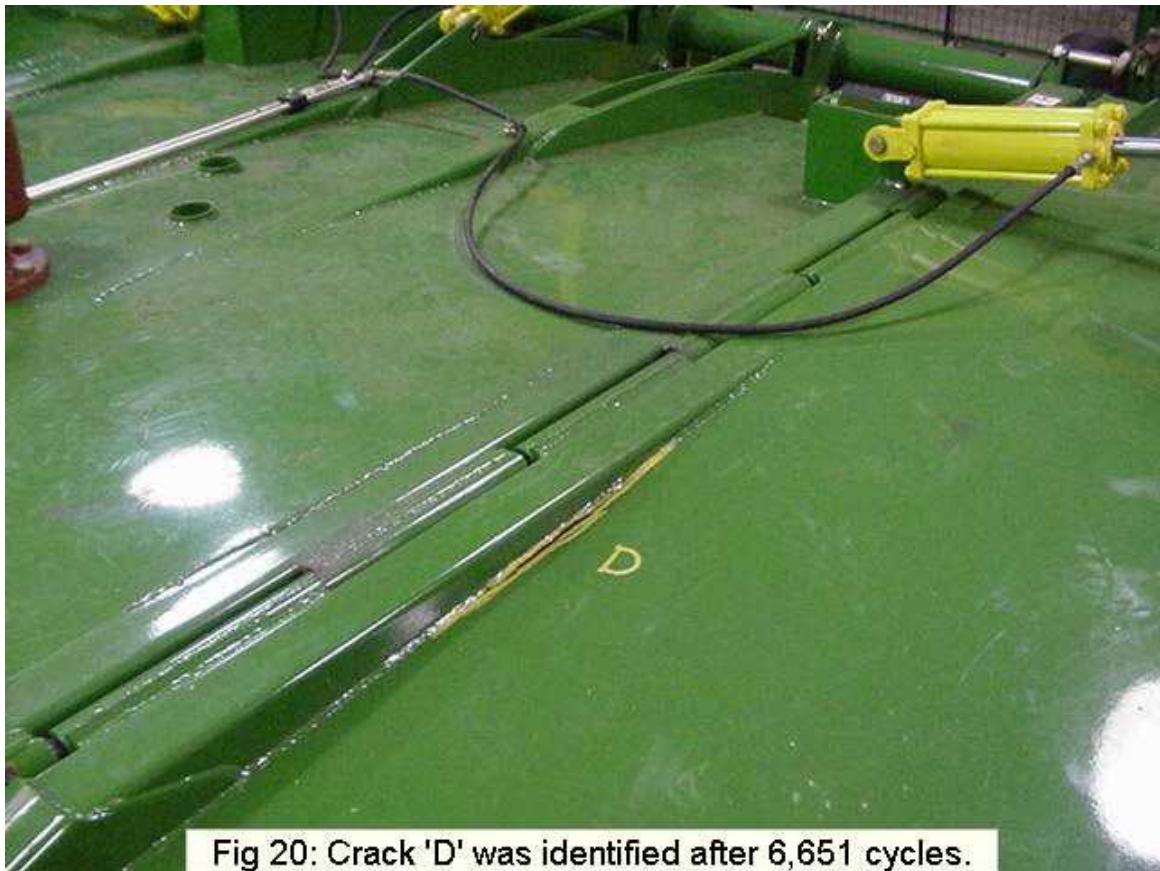
Figure 10 – Failure on Wing Cutter Top Deck
