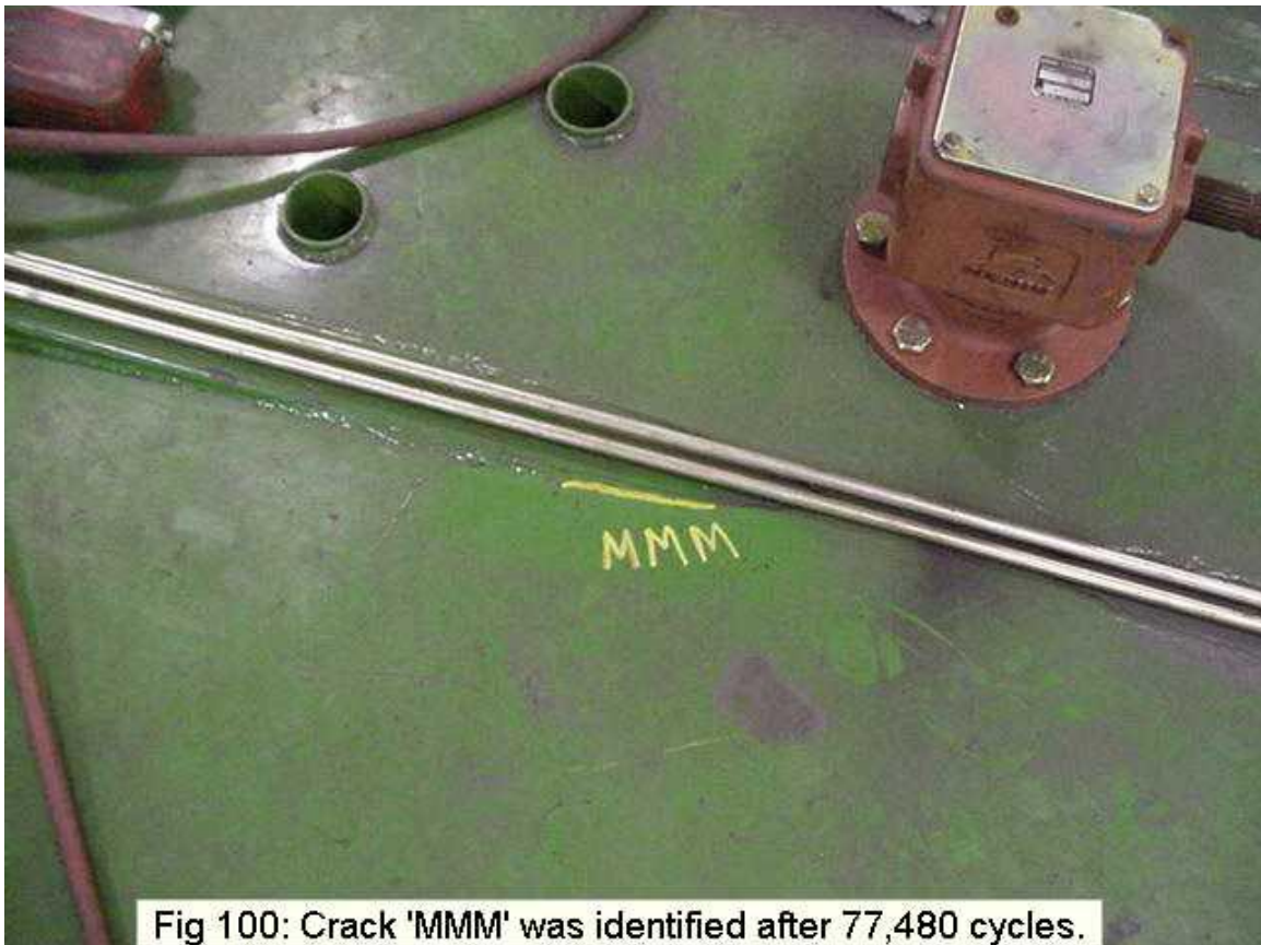
Figure 4 – Failure on top deck of Centre Cutter
