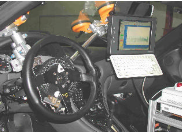
Instrumentation on the vehicle and recorded driver inputs during the test
