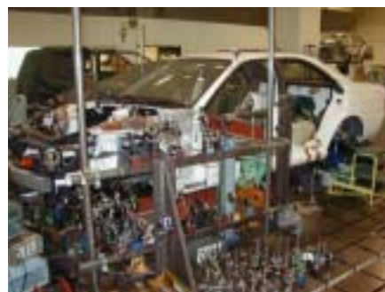
Fig.10 Bench test of body structure
