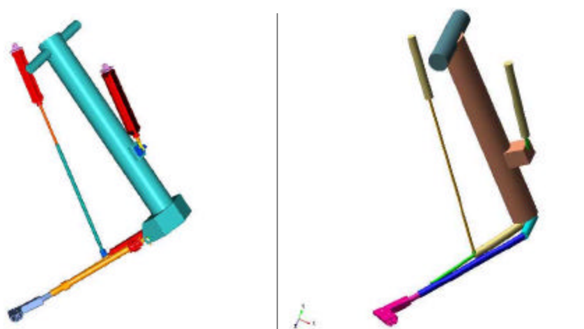
Figure 5. An I-DEAS (left) and corresponding ADAMS model (right) of the robot.
