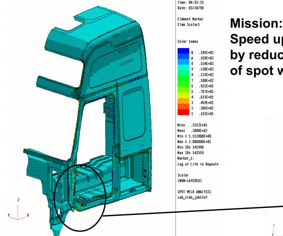
Speed up cab production by reducing total number of spot welds by 10%
