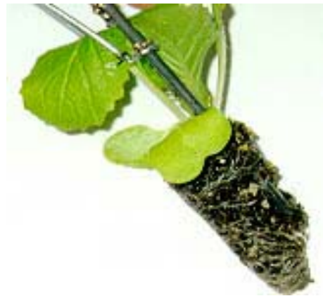
Fig. 21. Pick-up pin inserted to the upper of the seedling
