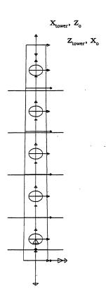
Each pair of parts in the tower is connected by one of the special WT tapered beam FIELD elements, running between the part centers-of gravity. The bottom-most part is connected to ground using a half-length tapered beam element. This is shown in the following figure.
