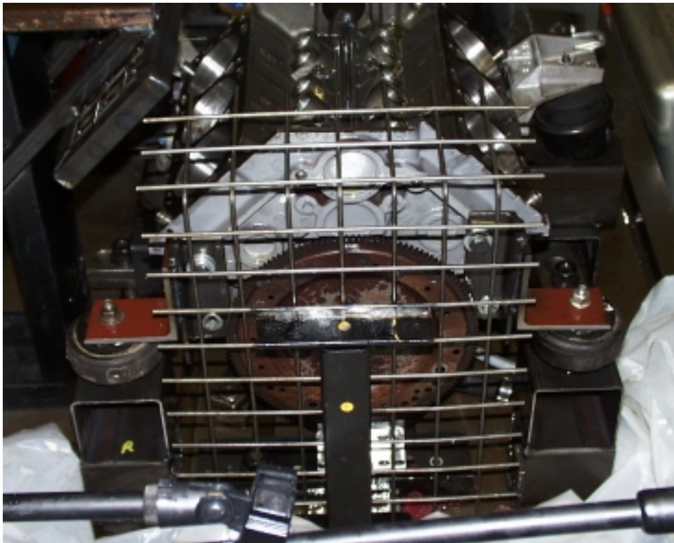
Figure 8. Two modified mounts at the transmission site
