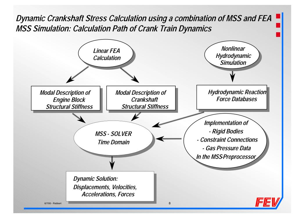
Dynamic Crankshaft Stress Calculation using a combination of MSS and FEA MSS Simulation: Crank Train Model
