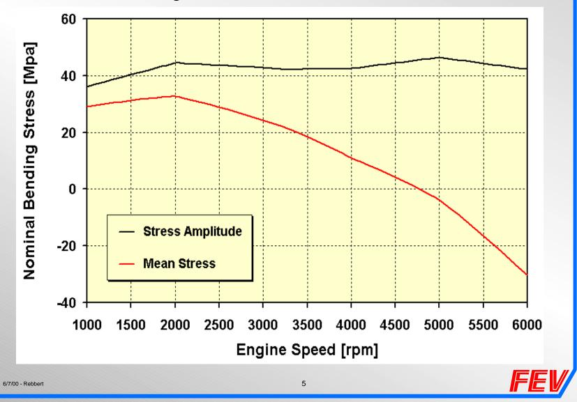
Dynamic Crankshaft Stress Calculation using a combination of MSS and FEA Traditional Procedure: FE-Analysis of Stress Concentration Factor
