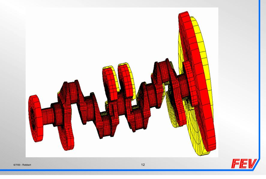
Dynamic Crankshaft Stress Calculation using a combination of MSS and FEA Comparison between traditional and new calculation method
