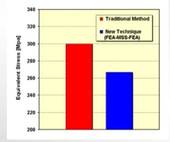
The additional safety margin detected by the new, more realistic method is about 12% at 6000 rpm, full load.
