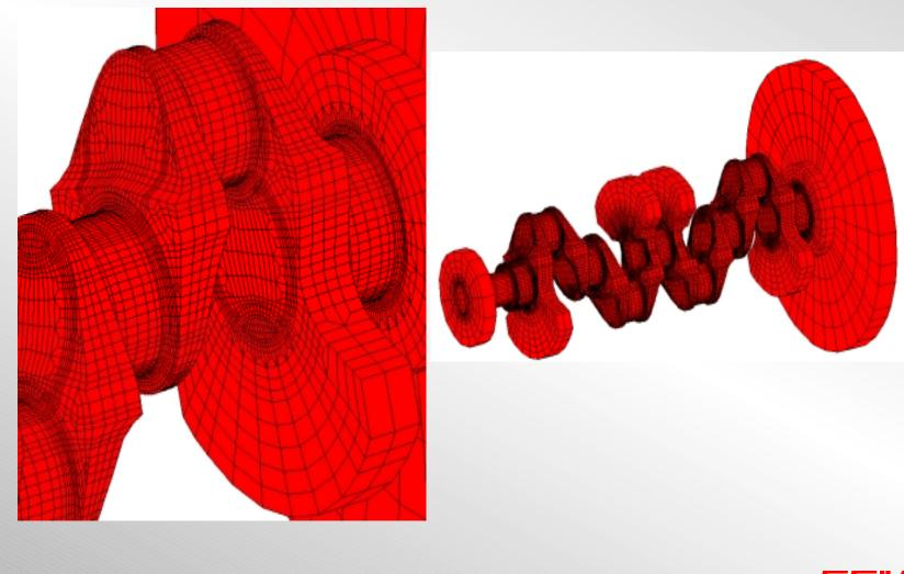
Dynamic Crankshaft Stress Calculation using a combination of MSS and FEA Recoupling of MSS Results to the FE-Analysis:
