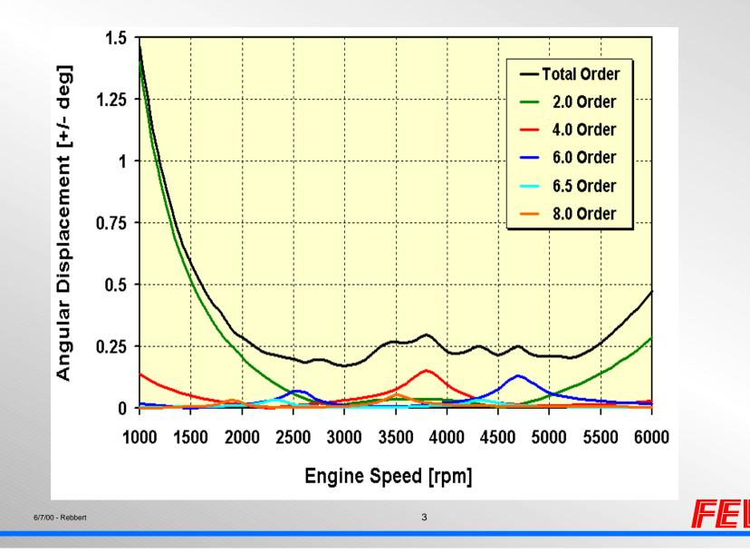
Dynamic Crankshaft Stress Calculation using a combination of MSS and FEA Traditional Procedure: Nominal Torsional Stress referred to the Crank Pin
