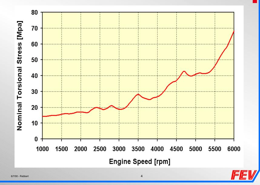
Dynamic Crankshaft Stress Calculation using a combination of MSS and FEA
