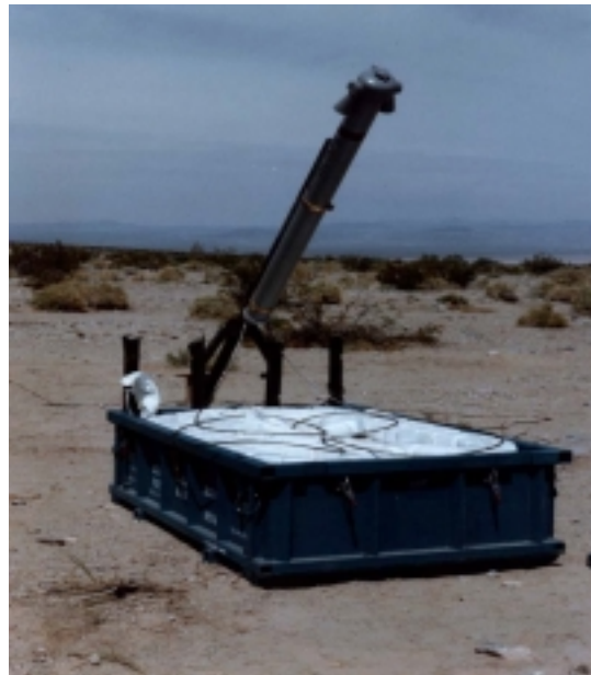
Figure 11. M58 system in Shipping Container
