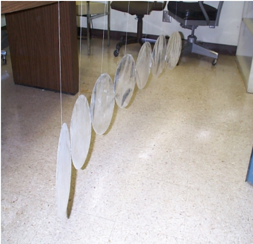
Figure 5. Solar Sail 6-Ring Model: Air Damping Test Set up
