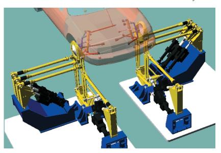
dation process so difficult are eliminated. Virtual sensors can be placed in the same location on the model as on the physical test article. The same analysis techniques are then used to validate the model. A validated model is a powerful tool as explained below.
