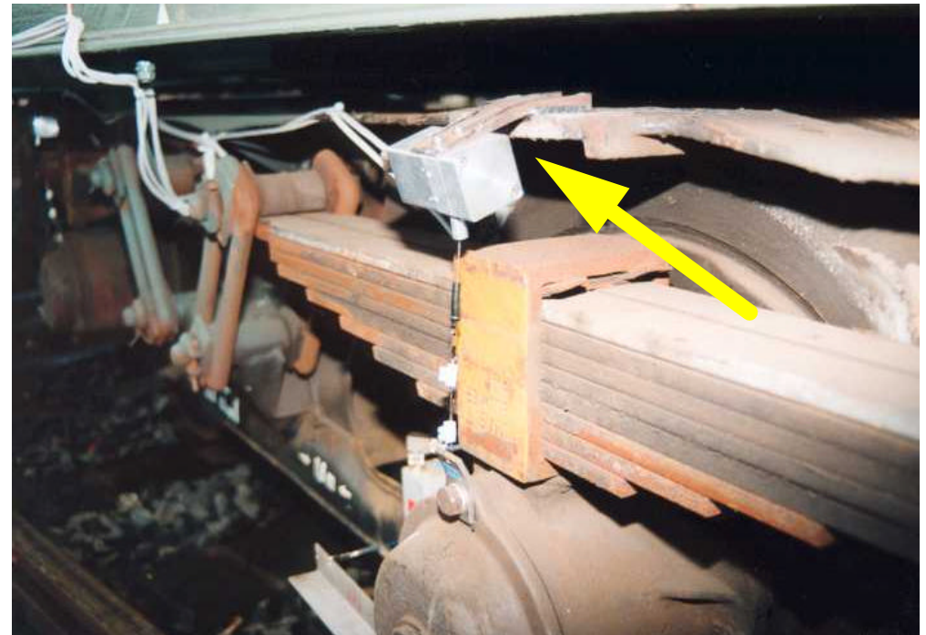
Demage of a sensor
