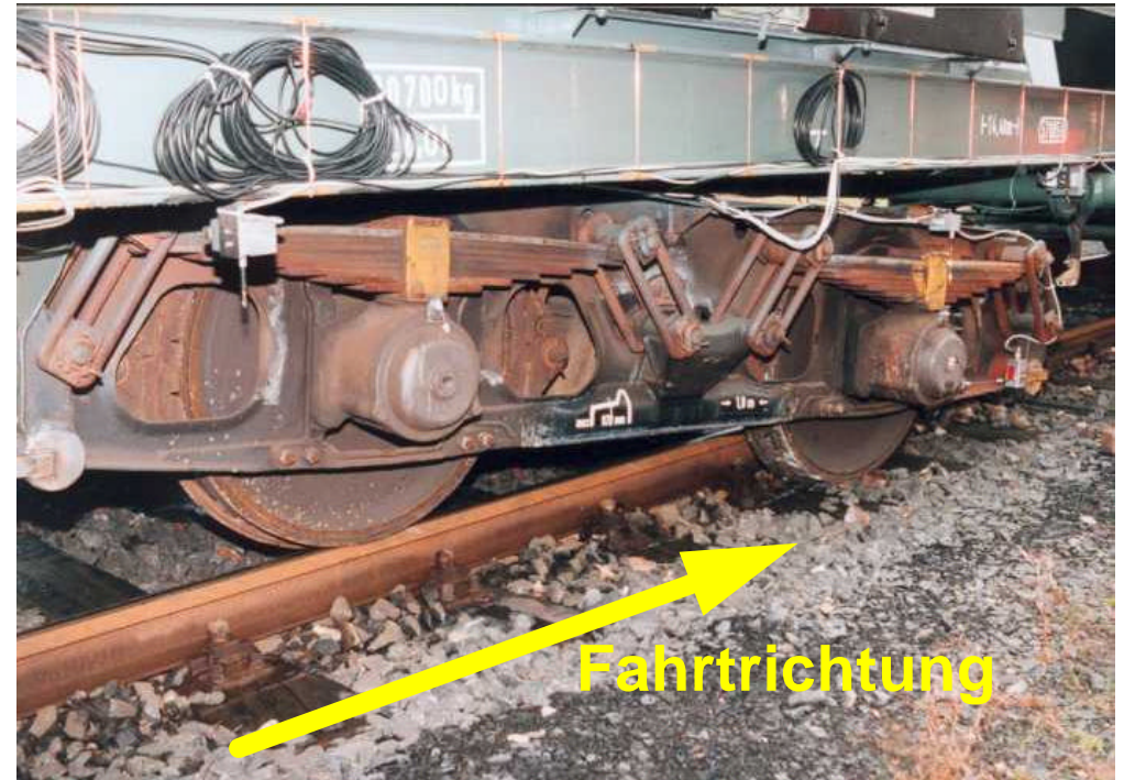
Derailed bogie (43 km/h)
