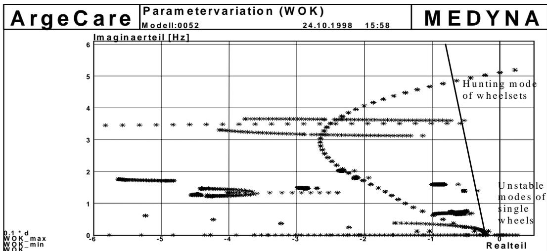
Fig 2: Root loci of the tram model for equivalent conicity 0.2
