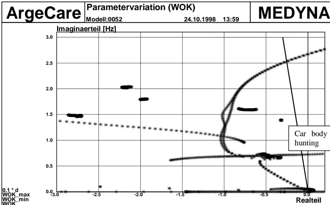
Fig 4: Root loci of the tram model for very low equivalent conicity (0.02)
