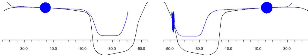
Fig 6: Flanging situation of wheels or wheelsets for hunting modes as represented in RSGEO
