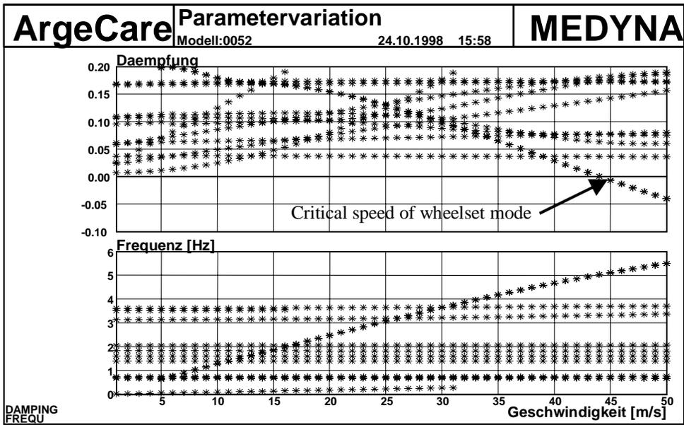
Fig 3: Frequency-damping function of the tram model for equivalent conicity 0.2
