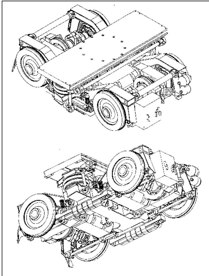
*Figure 1a: motor bogie*
