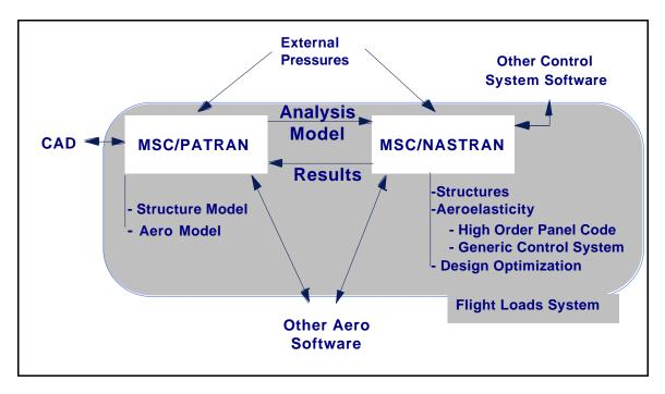
In basic terms, MSC/FlightLoads and Dynamics provides the ability to start with native CAD geometry and define an aeroelastic environment with coupled structural and aerodynamic models. This facilitates the definition and evaluation of the appropriate rigid aerodynamic pressure distributions and aeroelastic influence coefficients to generate the external loads on the vehicle. All of these steps are driven from a graphical system.
