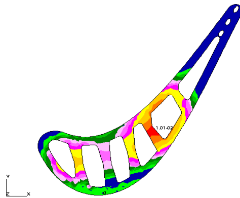
Figure 6b. Cumulative creep damage at each element demonstrates proportion of life used
