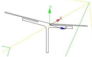
When a new orientation definition has been defined pressing the Preview Axis Definition Button will update the display so the User can evaluate the effect of the modification.
