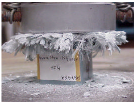
FIGURE 1 QUASISTATIC CRUSHING OF A SQUARE PULTRUDED GLASS/POLYESTER TUBE
