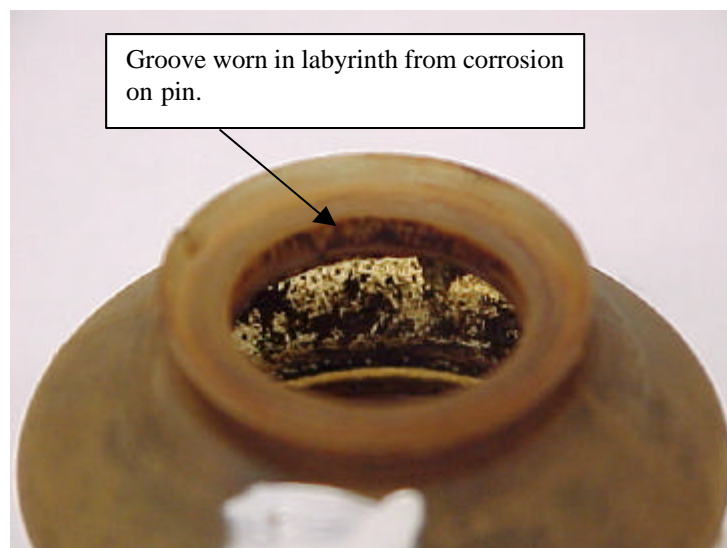
Fig. 1b Ball joint sealing boot failure: excessive wear in labyrinth.
