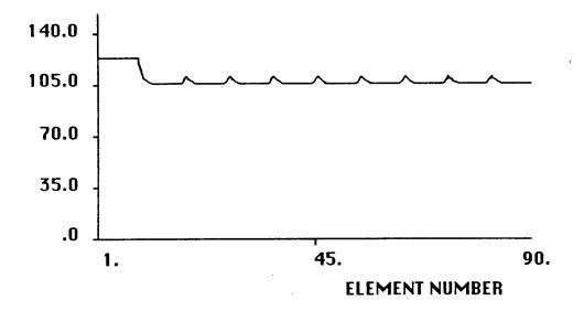
Spherical Shell: Von Mises Stress Levels, Pressure Loading
