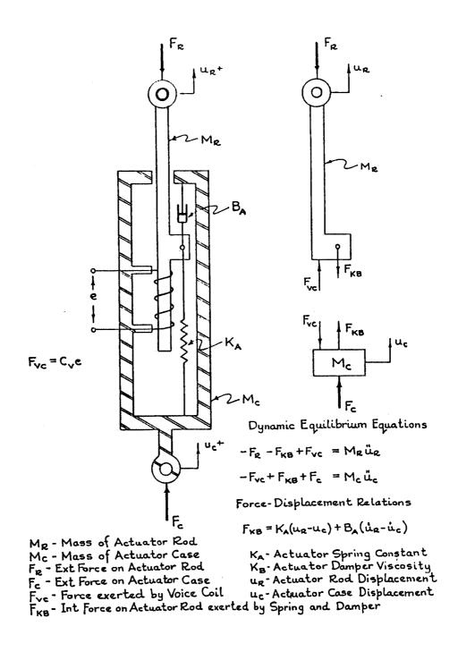
Figure 2 - Detailed Sketch of Voice-Coil Actuator (VCA)
