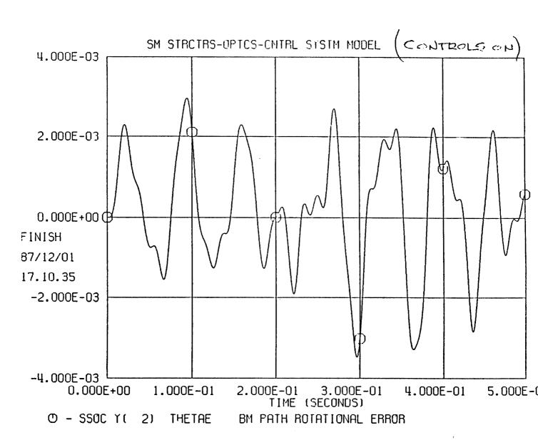
Figure 5 - Laser Beam Angular Error vs Time (Controls ON) as Calculated by TIMRSP
