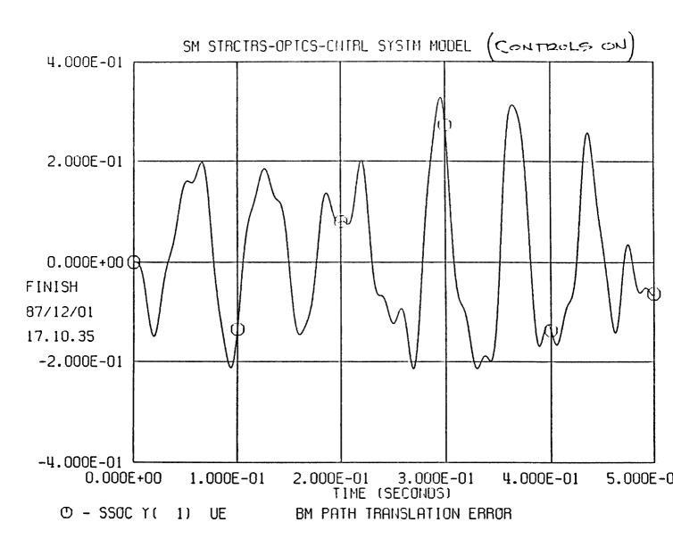
Figure 3 - Laser Beam Path Translational Error vs Time (Controls ON) as Calculated by TIMRSP
