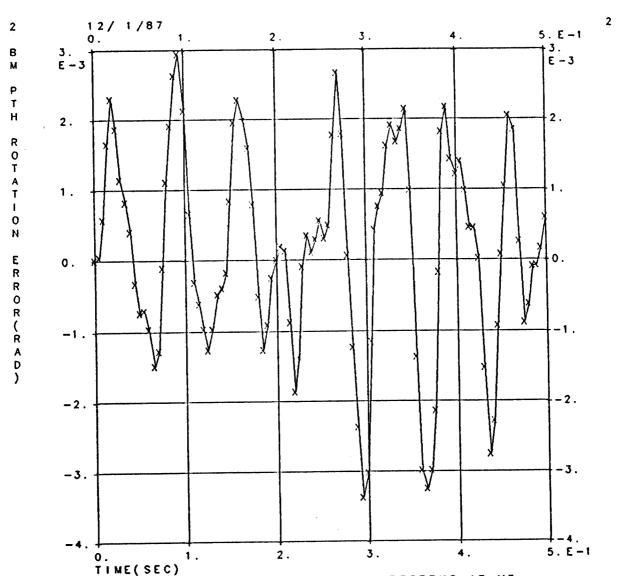
BEAM PATH ROTATION ERROR VS. TIME FOR DSTRBNC AT M7 SIMULATION OF SMALL STRCTRS-OPTCS-CNTRL SYSTEM DIRECT METHOD TRNSNT RSPNS (CNTRLS ON)
