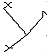
Figure 18: Deformed shape of flexible golf club
