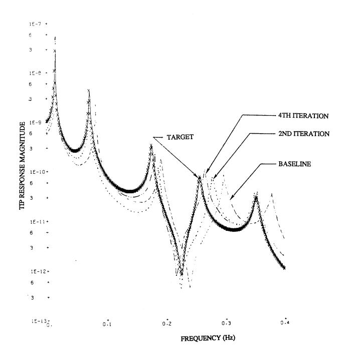
Fig.2. Comparative Iteration FRF Curves
