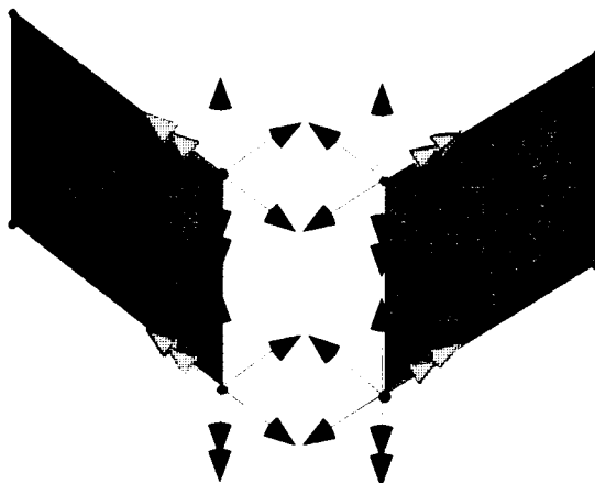
Figure 1: Kinematic dof at the intersection between two CQUAD4 elements.
