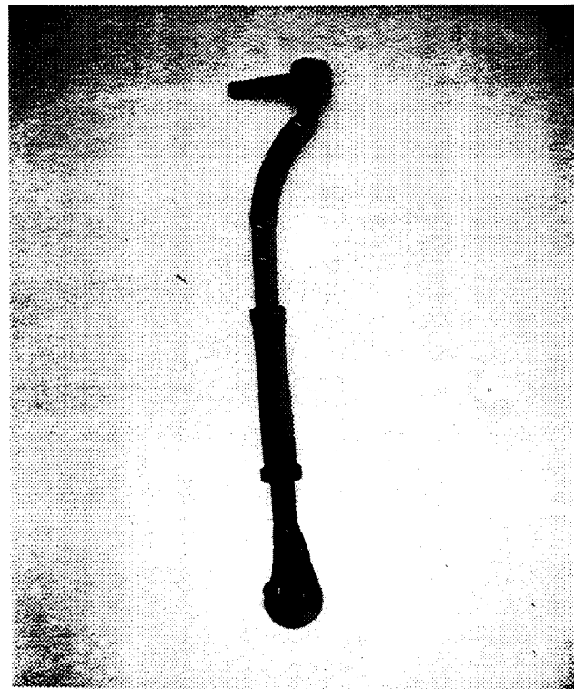
Figure 5. Tie rod sample - Before and after the buckling test.
