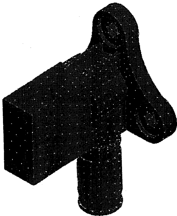
Fig. 7 Finite Element Model Of Accelerometer
