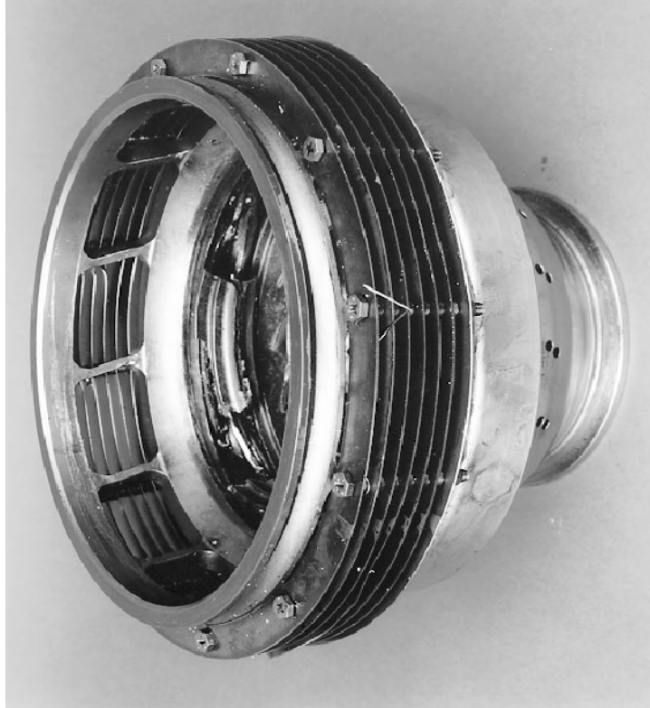
Inlet housing after rim and blade test
