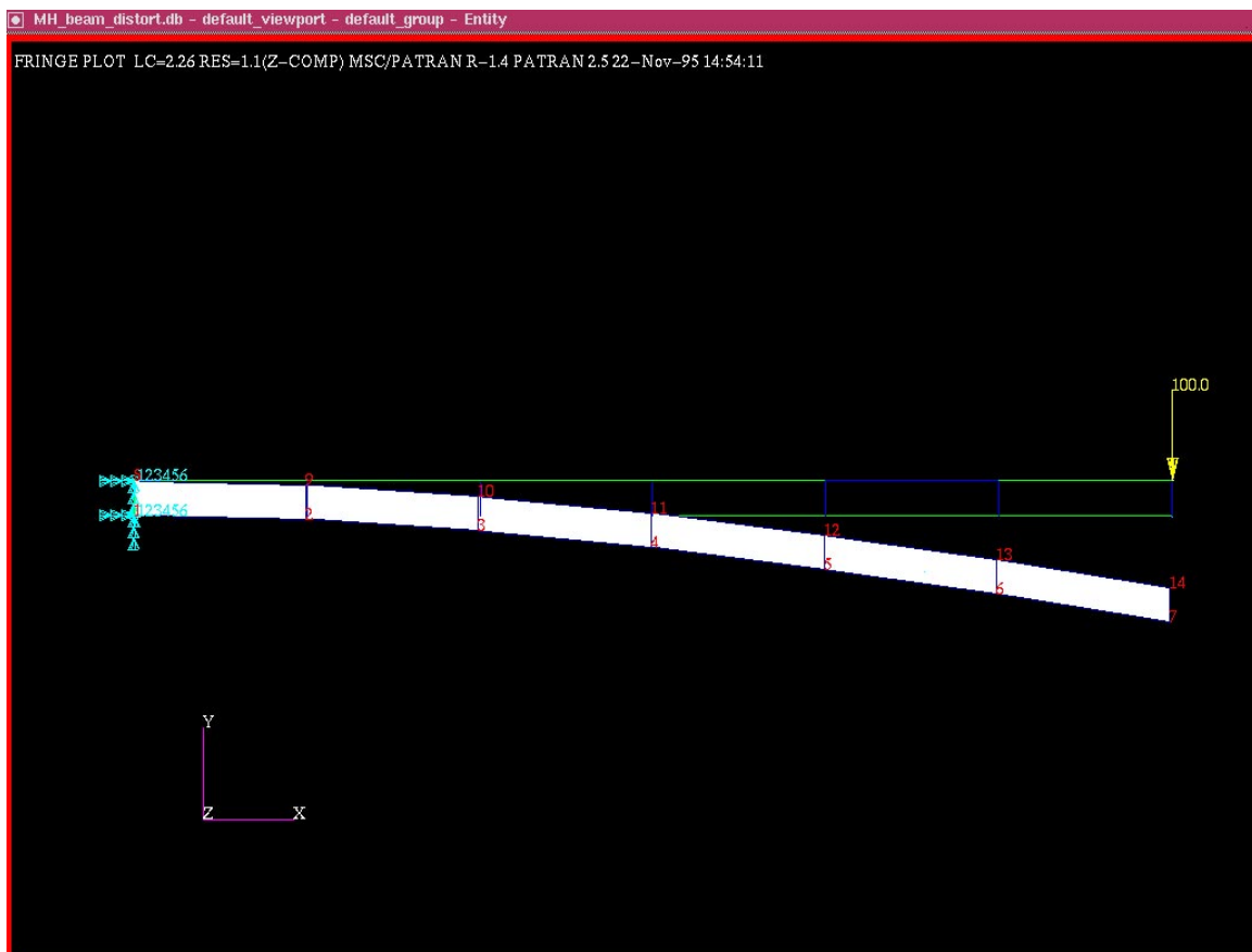
FIGURE 3 VISUALIZATION OF DISPLACEMENT RESULTS READ BACK INTO PATRAN
