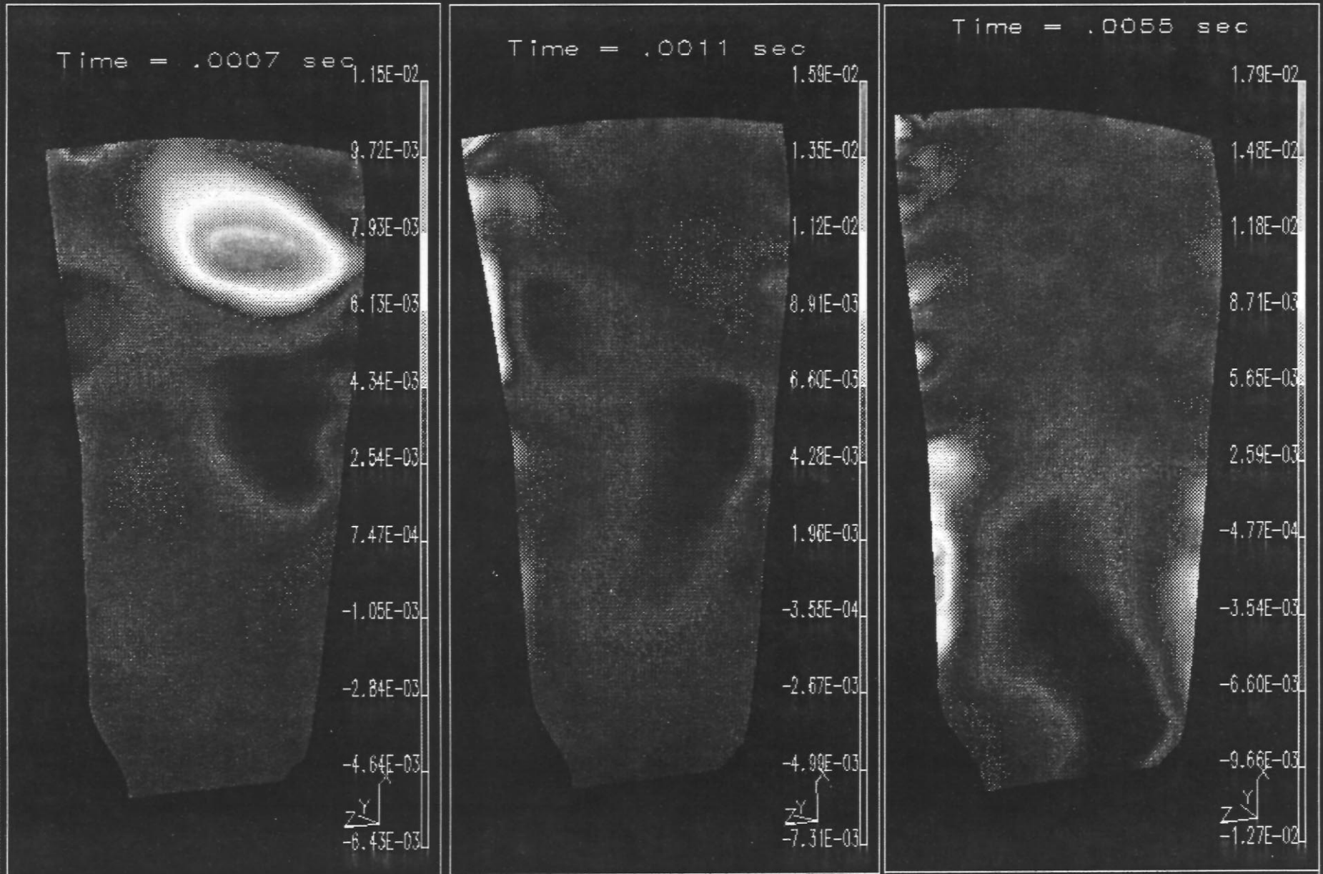
FIGURE 5: BLADE STRAINS DURING AN FOD EVENT
