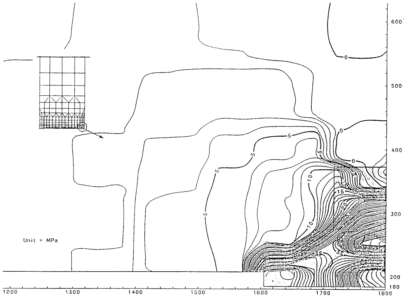
FIG. 14: CONTOUR OF LONGITUDINAL NORMAL STRESS ( \sigma_z ) AT \theta = 0^\circ LOAD CASE 3 = BENDING MOMENT
