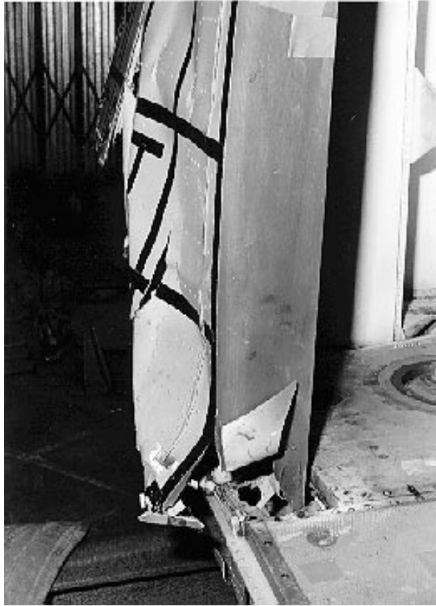
Fig. 11 - Vertical drop test- Failure of starboard main liftframe.
