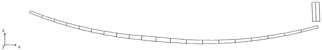
Figure 4. MDI/ADAMS Model of a Single Taper Leaf with Shackle in the Rear.
