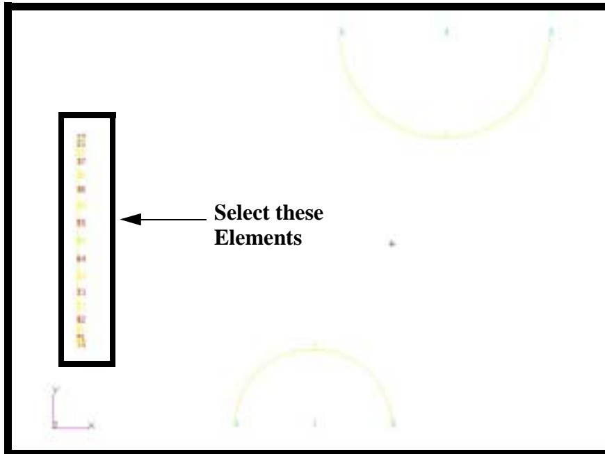
Figure 12.4 - Bar elements to sweep into surface elements
