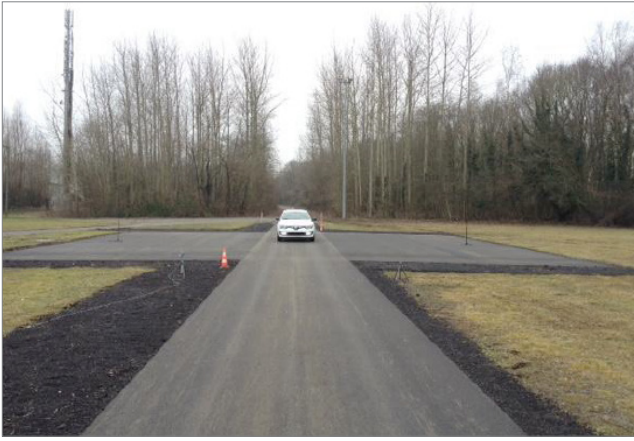
Pass-by Noise Measurement Setup
